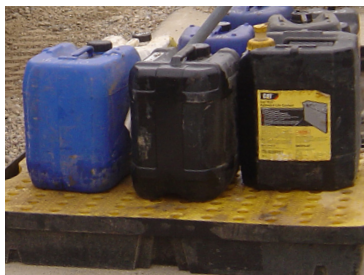
Figure 1: Containers should be stored on pallets which incorporate a sump
