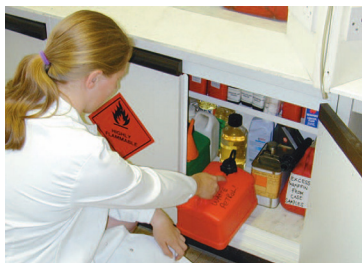
Figure 2: Small containers in the workplace should be stored in a purpose-built flammable liquid cabinet
